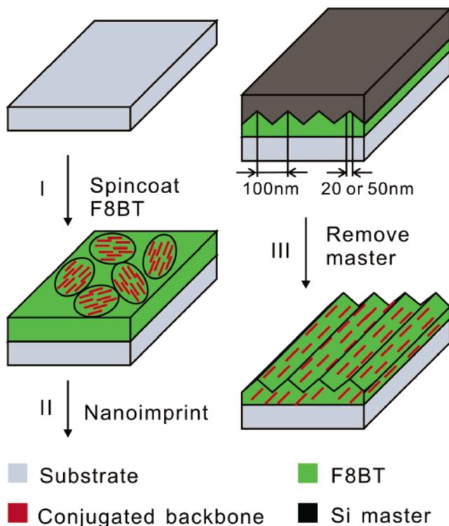
**Figure 1.** Schematic process of aligning F8BT by nanoconfinement.
